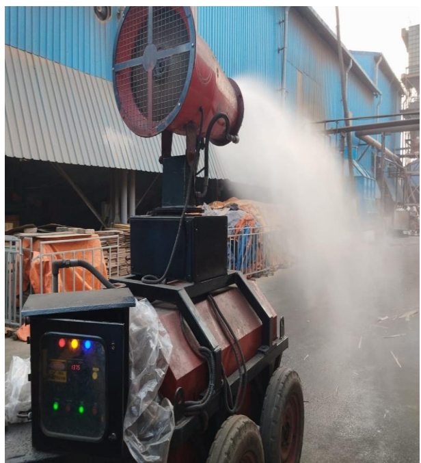
Photo: Water mist sprayer for proper dust suppression on the road and inside the plant
