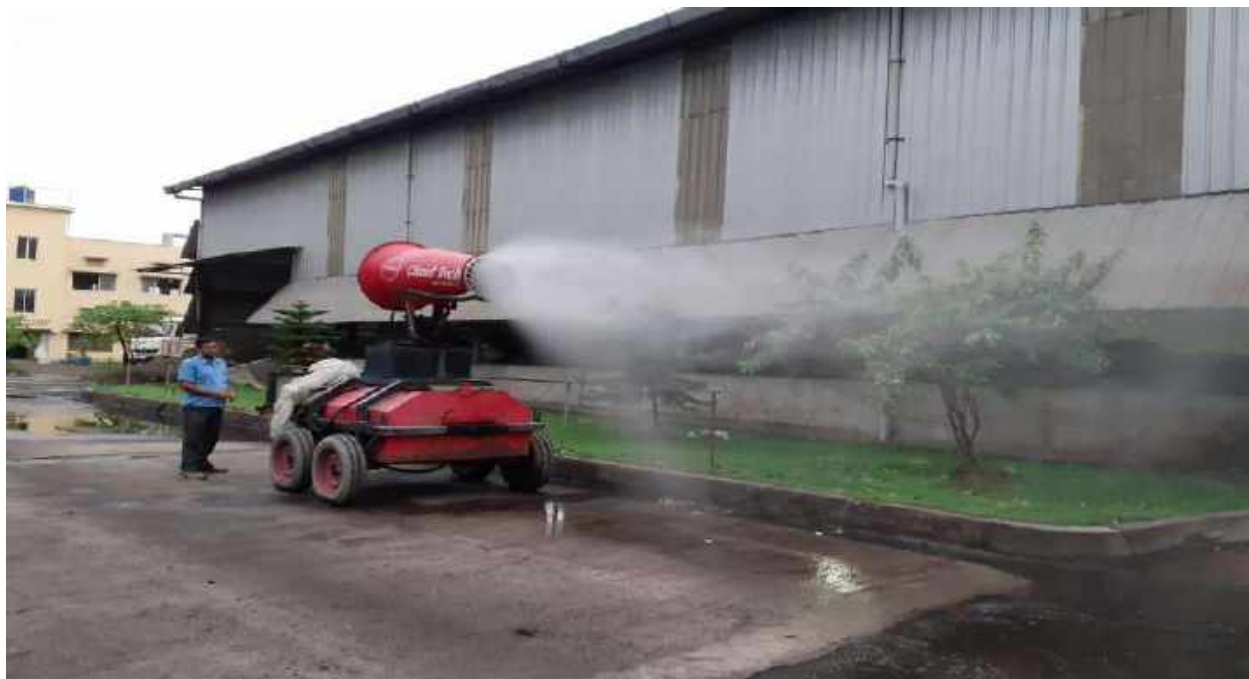
Photo: Water mist sprayer for proper cleaning of road
